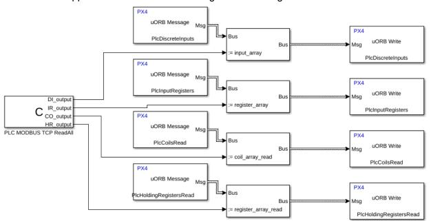
Lower Section: Demonstration of reading the uORB topics that are connected to the MODBUS TCP Client
